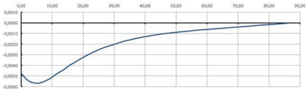
**Fig. 12.** Distribution diagram of vertical displacements along the third cross-section (Vertical axis represents values of displacements, horizontal axis – distance from the external wall of the pit)
