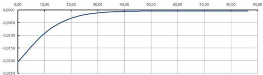
**Fig. 11.** Distribution diagram of horizontal displacements along the third cross-section (Vertical axis represents values of displacements, horizontal axis – distance from the external wall of the pit)
