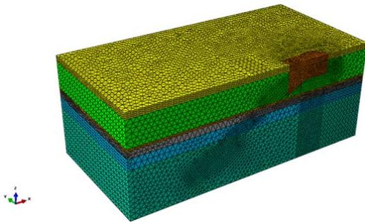
**Fig. 3.** Overview of the finite-element model of soil mass, which is containing the discussed object
