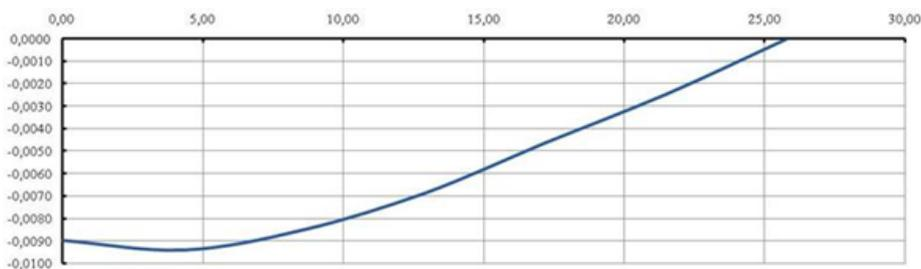
Fig. 10. Distribution diagram of vertical displacements along the second cross-section (Vertical axis represents values of displacements, horizontal axis – distance from the external wall of the pit)
