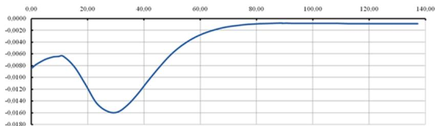
**Figure 7.** Distribution diagram of horizontal displacements along the first cross-section (Vertical axis represents values of displacements, horizontal axis – distance from the external wall of the pit)
