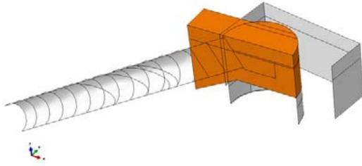
**Fig. 1.** Mutual orientation of the grouting zone, slurry wall and the tunnel lining
