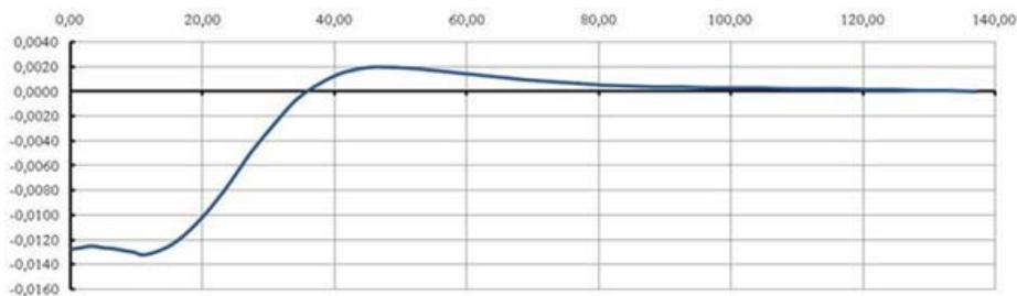
Figure 8. Distribution diagram of vertical displacements along the first cross-section (Vertical axis represents values of displacements, horizontal axis – distance from the external wall of the pit).
