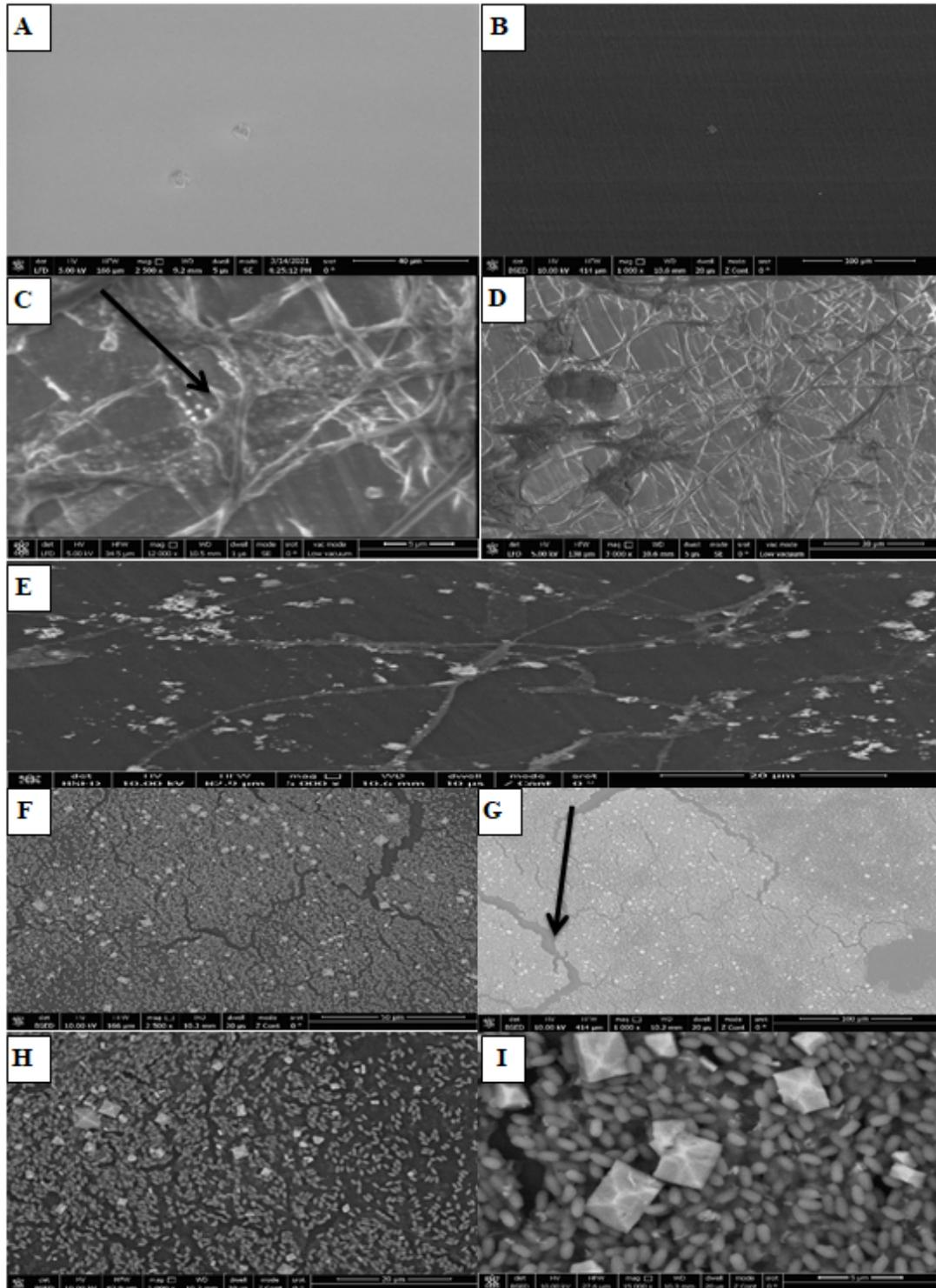
**Picture 6.** SEM analysis of (LDPE) film, control (6A, 6B), (LDPE) treatment with *F. equiseti* (6C, 6D, 6E), and LDPE treatment with *B. parabravis* (6F, 6G, 6H, 6I)
