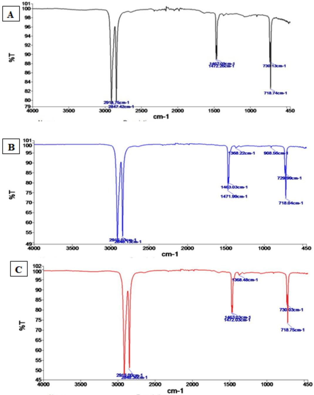
Fig. 3. FTIR analysis, (3A) control (LDPE film only), (3B-3C) (LDPE) film treatment with *F. equiseti* and *B. parabrevis*, respectively
