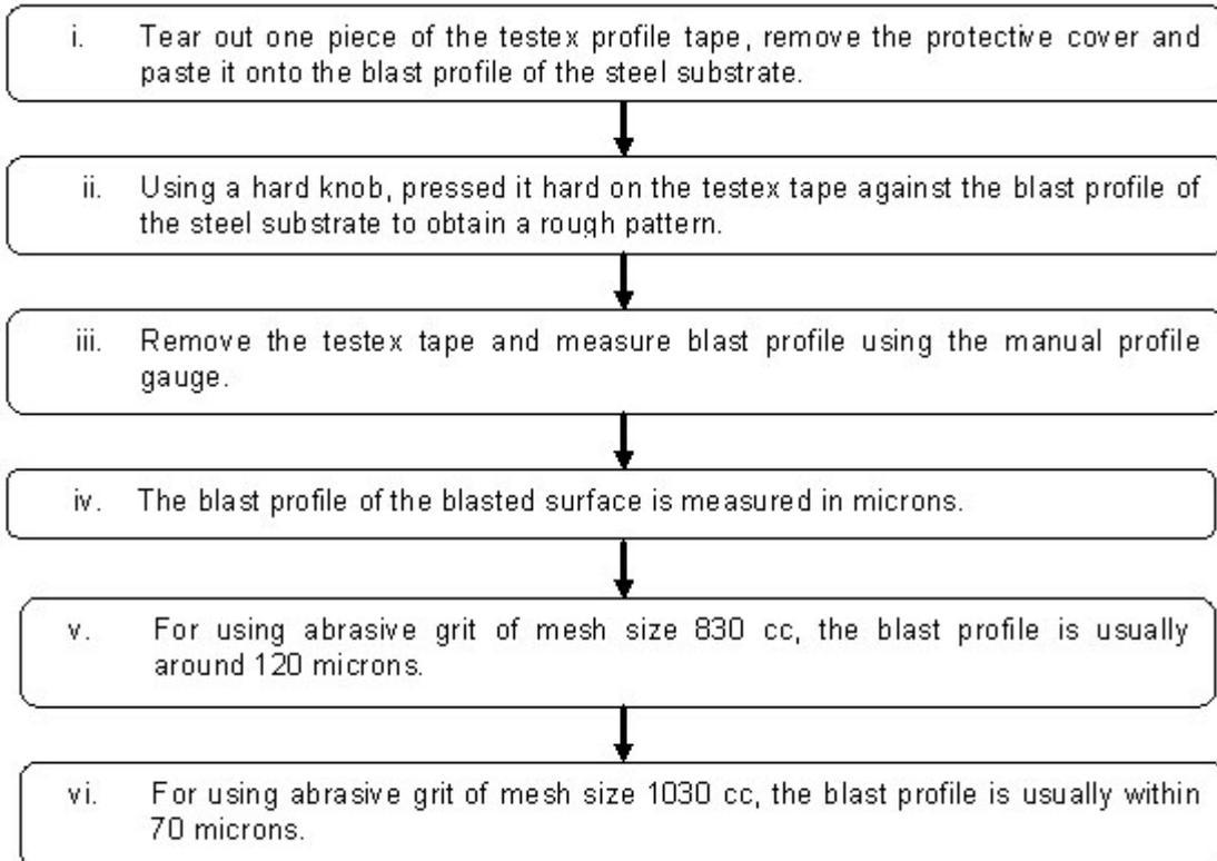
Fig. 3: Flow chart of blast profile measurement by testex profile tape
