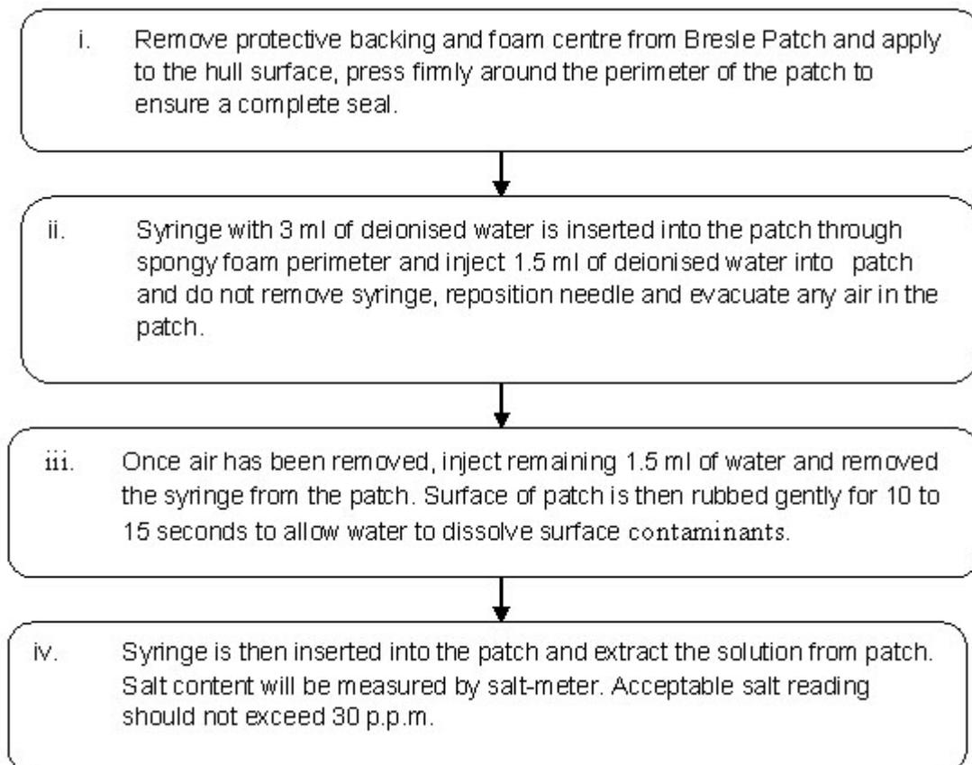
Fig. 2: Flow chart of salt test measurement by “Bresle kit sample”
