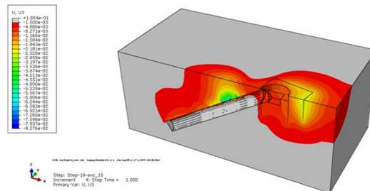
**Fig. 6.** Zone of intensive vertical displacements (up to 0.0010...0.0015 m) (with specified characteristic cross-sections 1, 2 and 3).
