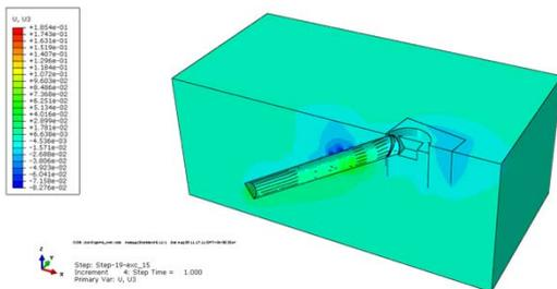
**Fig. 5.** Diagram of resulting vertical displacements (with specified characteristic cross-sections 1, 2 and 3)
