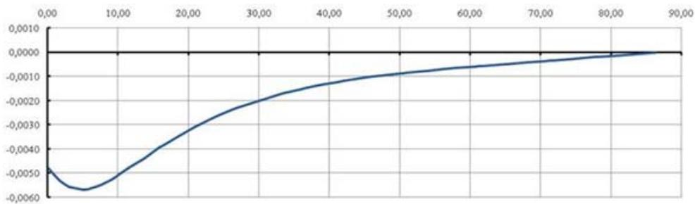
**Fig. 12.** Distribution diagram of vertical displacements along the third cross-section (Vertical axis represents values of displacements, horizontal axis – distance from the external wall of the pit)
