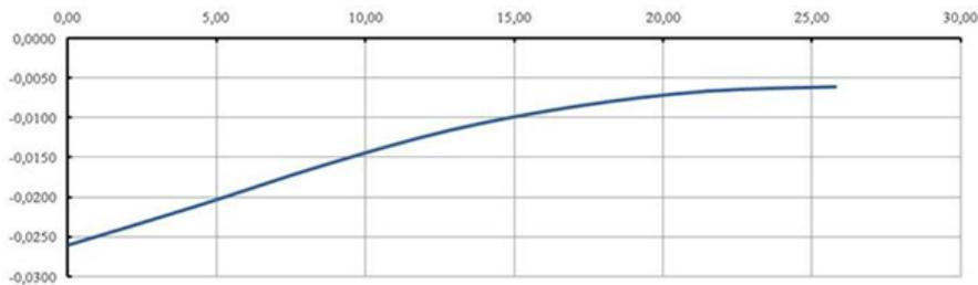
Fig. 9. Distribution diagram of horizontal displacements along the second cross-section (Vertical axis represents values of displacements, horizontal axis – distance from the external wall of the pit)
