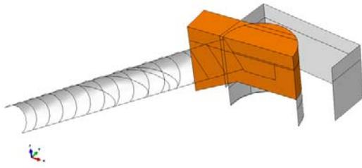
**Fig. 1.** Mutual orientation of the grouting zone, slurry wall and the tunnel lining
