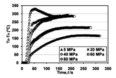
Fig. 3. The difference in temperature between the internal and external surfaces of the mold with the passage of time and increasing the process pressure
