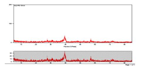
Fig. 1. XRD test chart of heat treated glass at 600C
