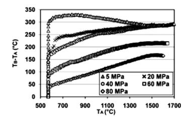
Fig. 4. The difference between the internal and external surface of the die with increasing process temperature at different pressures
