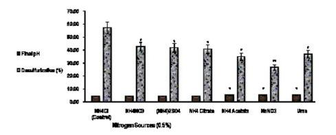
(values were expressed as Mean  $\pm$  SEM, where n = 6; \* p < 0.05, \*\* p < 0.01 when compared to control) Fig. 3. Effect of different nitrogen sources (0.5%) on desulfurization of Coal by the mutant *Thiobacillus ferrooxidans* X<sub>200</sub>
