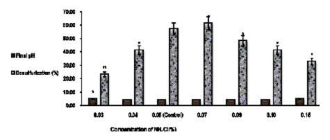
(values were expressed as Mean  $\pm$  SEM, where n = 6; \* p < 0.05, \*\* p < 0.01 when compared to control) **Fig. 4.** Optimization of NH<sub>4</sub>Cl for desulfurization of Coal by the mutant *Thiobacillus ferrooxidans* X<sub>200</sub>
