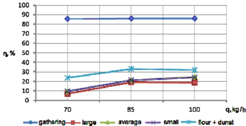
Fig. 8. Dependency of extraction factor  $\eta$  (%) from load (q), kg/h
