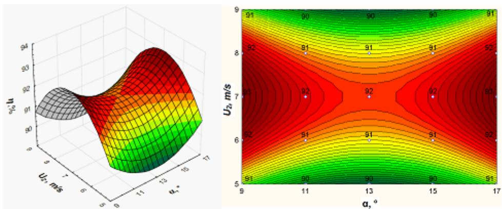
**Fig. 3.** Influence of factors  $X_1, X_3$  (a) response surface; (b) two-dimensional section
