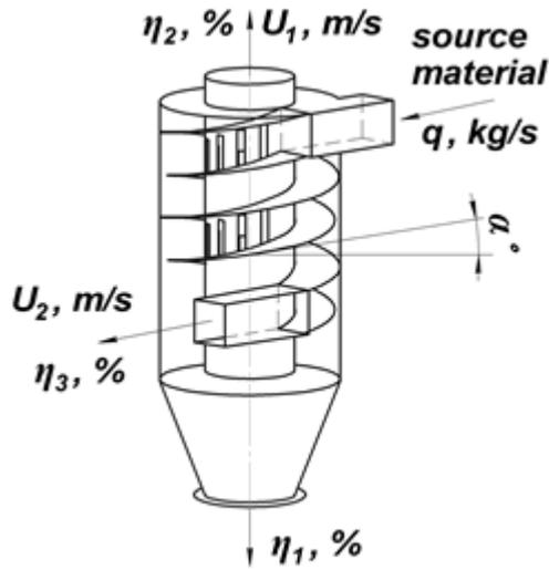
**Fig. 1.** Factors influencing the grain milling product separation in pneumatic screw channel
