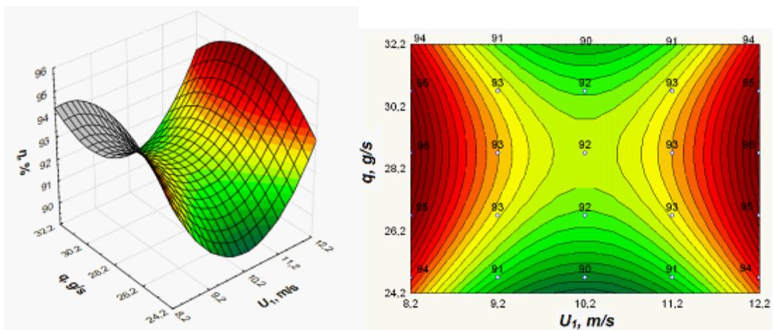
Fig. 6. Influence of factors  $X_2X_4$  (a) response surface (b) two-dimensional section.
