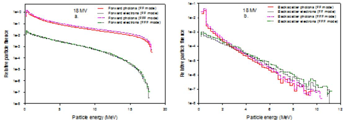
**Fig. 8.** The fluence spectra of 18 MV reached to the upstream surface of the BMC in the case of the FF and FFF mode, a. for the forward directed photons and electrons for each field size, b. for the backscattered photons and electrons for the  $0.5 \times 0.5$  cm<sup>2</sup> field size. The spectra have been normalized to the maximum of the forward photon fluence in the case of the FF mode for the  $0.5 \times 0.5$  cm<sup>2</sup> field size.
