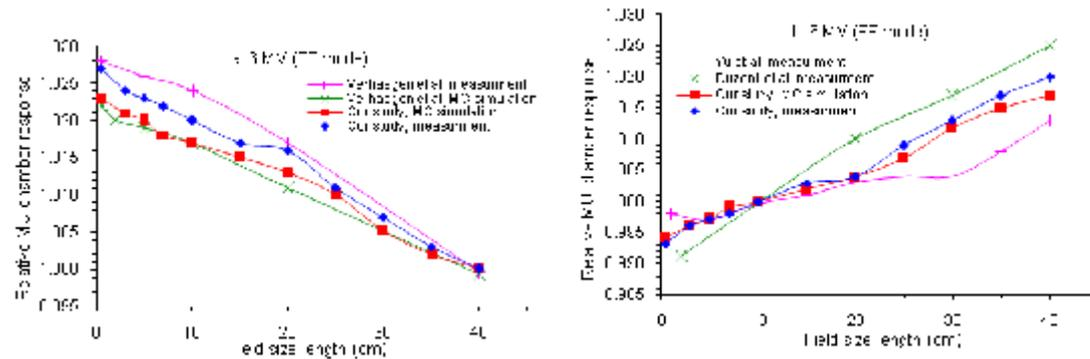
**Fig. 4.** The variation of relative BMC response as a function of field size for 6 MV photon beam of the conventional Linac (FF mode). All data are normalized to a) the  $40 \times 40$  cm<sup>2</sup> field size, b) the  $10 \times 10$  cm<sup>2</sup> field size.
